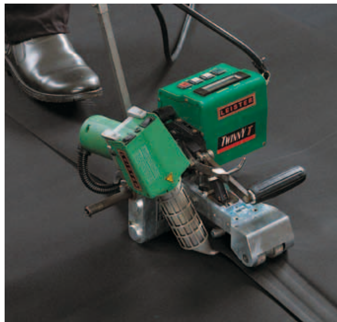
Seams with air pressure test channels are produced with dual hot wedges. The dual wedge provides easy air pressure testing of seams both immediately after installation and after many years of service.
